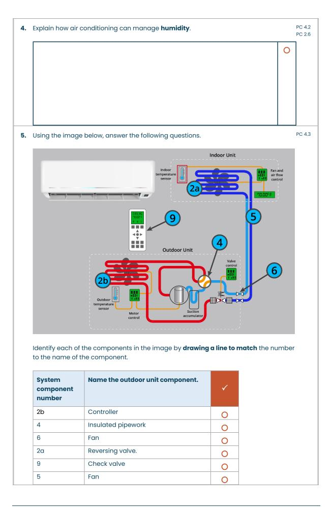
6. There are TWO (2) fans in the image. Draw a line to Match the number of the fan with PC 4.3 the description of its function.
